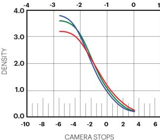
"0" on the x-axis represents normal exposure of an 18-percent gray card in the red, green, and blue layers of this film. A white card is  $2\,\%$  stops higher than normal exposure. A 3-percent black card is  $2\,\%$  stops below normal exposure.
