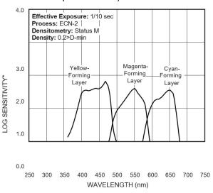
\*Sensitivity = reciprocal of exposure (erg/cm²) required to produce specified density
