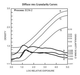
Read with a microdensitometer, using a 48-micrometre aperture.
